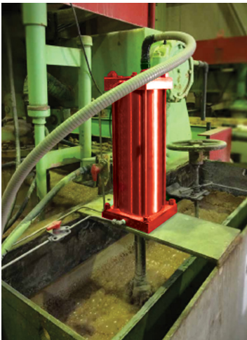
8" Bore Stainless Steel HP Series with remote positioner in a potash plant.
