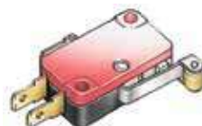
Type G / MG (2) SPDT Mechanical Gold-Plated Contacts 1 amp @ 125 VAC 1 amp @ 24 VDC Minimum 1 mA
