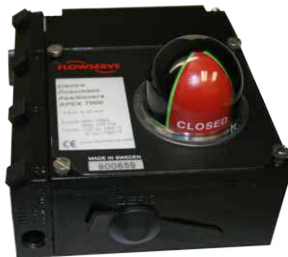
Electro-pneumatic Positioner Apex 7100 shown with weatherproof I/P housing and UltraDome indicator
