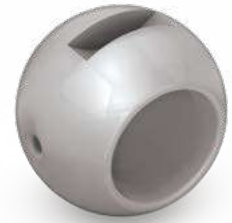
3 mm relief hole face the upstream
