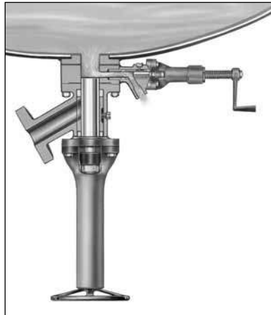
Fig. 2 - Drain Valve Open for Sample
